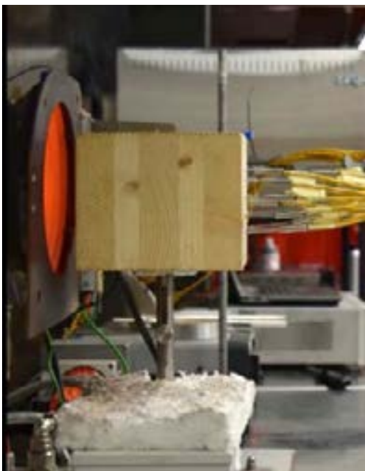
Figure 2: Radiant cone heater on CLT section with multiple thermocouples.
