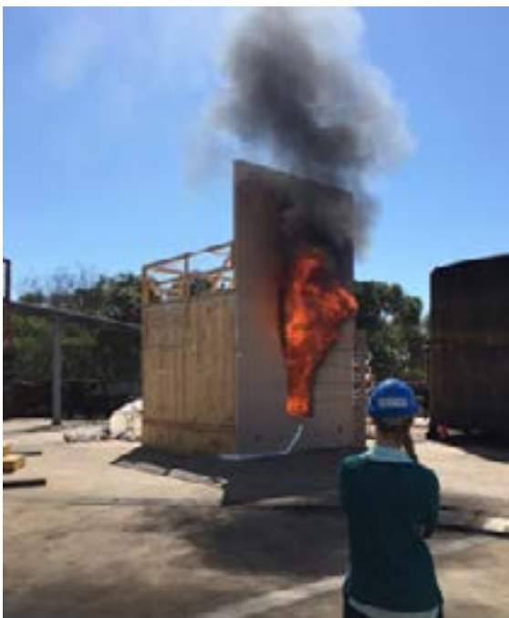
Figure 5: CLT enclosure and facade test.
