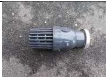
Suction Strainer (one-way valve)
