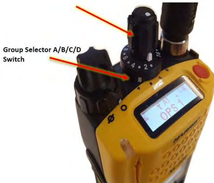
Example Shown: Group A, Channel 1: A1 Channel Name: OPS 1 NB: This screen does not show 'Zone'
