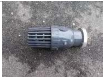
Suction Strainer (one-way valve)
